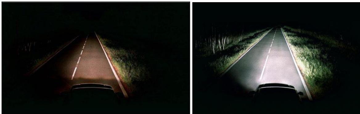
image 9 : Road visibility with Halogen (left) and Xenon (right) low beam
