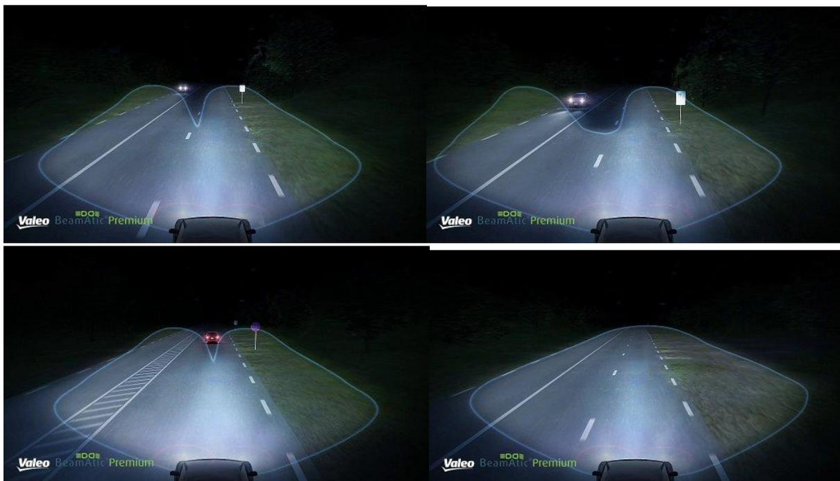
image 8 : Valeo BeamATIC® Premium beam schematics with an oncoming car (top left), car approaching (top right), with a preceding vehicle (bottom left) and full beam (bottom right)
