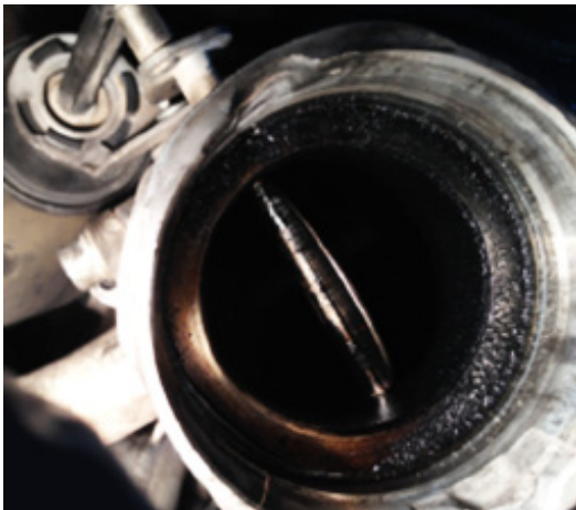
Fig. 3. Flap belonging to the exhaust-gas recirculation valve (EGR valve) coked
