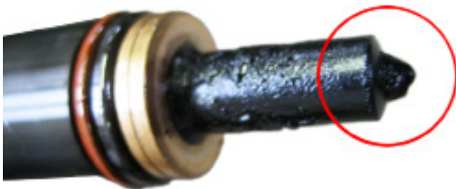
Fig. 3. Unit-injector element coked
